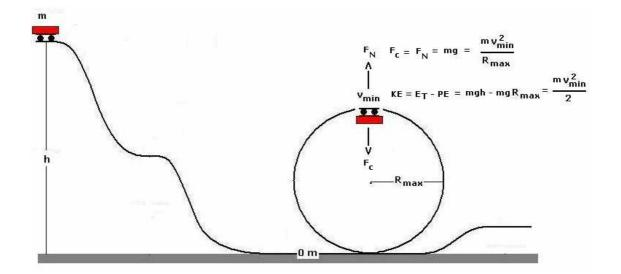
A roller coaster of mass **m** at rest at the top of a frictionless roller coaster track of height **h** descends to base level and then enters an inverted circular loop. Derive the equations for calculating the maximum permissible radius [ $\mathbf{R}_{max}$ ] of the inverted circular loop in order for the roller coaster to remain on the track and completely transit the loop.
